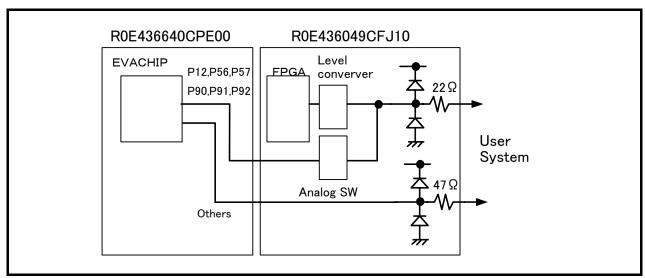
Figure 5 Connections of the R0E436049CFJ10
